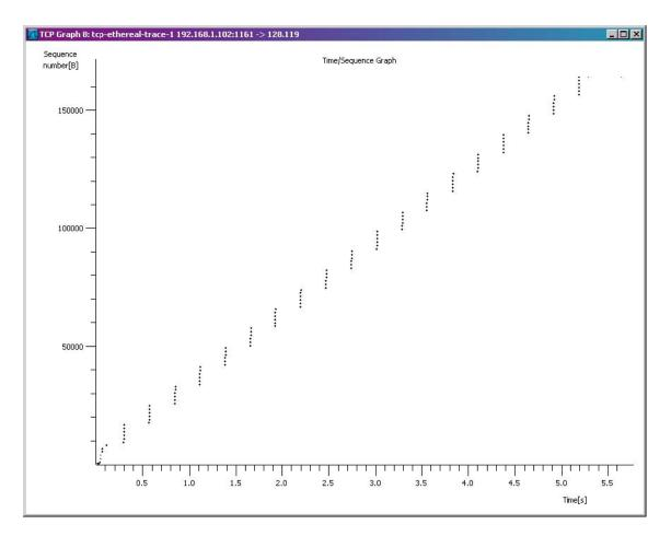
Here, each dot represents a TCP segment sent, plotting the sequence number of the segment versus the time at which it was sent. Note that a set of dots stacked above each other represents a series of packets that were sent back-to-back by the sender.
