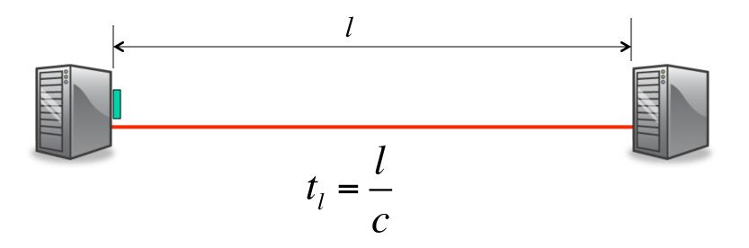
Example: A bit takes 5ms to travel 1,000km in an optical fiber with propagation speed 2 x 10<sup>8</sup> m/s.
