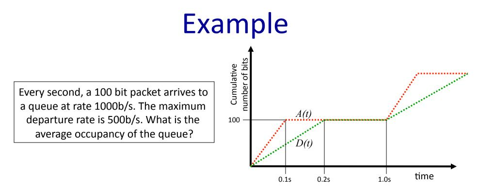
Solution: During each repeating 1s cycle, the queue fills at rate 500b/s for 0.1s, then drains at rate 500b/s for 0.1s. Over the first 0.2s, the average queue occupancy is therefore  $0.5 \times (0.1 \times 500) = 25$  bits. The queue is empty for 0.8s every cycle, and so average queue occupancy:  $\overline{Q}(t) = (0.2 \times 25bits) + (0.8 \times 0) = 5bits$
