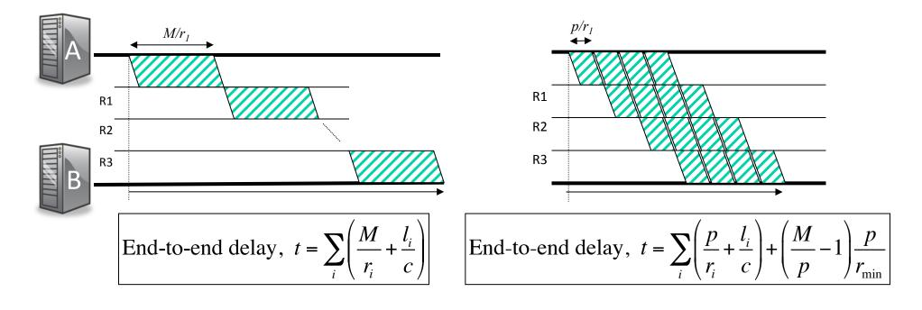
Breaking message into packets allows parallel transmission across links in a path, reducing end to end delay.
