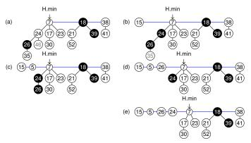
(a) The initial Fibonacci heap. (b) key 46 was decreased to 15. (3) The node becomes a root, and its parent (with key 24) gets marked. (c)–(e) the node with key 35 has its key decreased to 5. Its parent (key 26) is marked, and a cascading cut occurs. The node with key 26 is cut from its parent and becomes an unmarked root in (d). Another cascading occurs since node with key 24 is marked too. This node gets cut from its parent and made an unmarked root in (e). At this stage, cascading stops.
