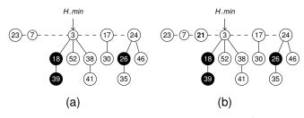
(a) A Fibonacci heap H. (b) Fibonacci heap H' produced after inserting the node with key 21 in H. The node becomes its own heap-ordered tree and is then added to the root list, becoming the left sibling of the root.
