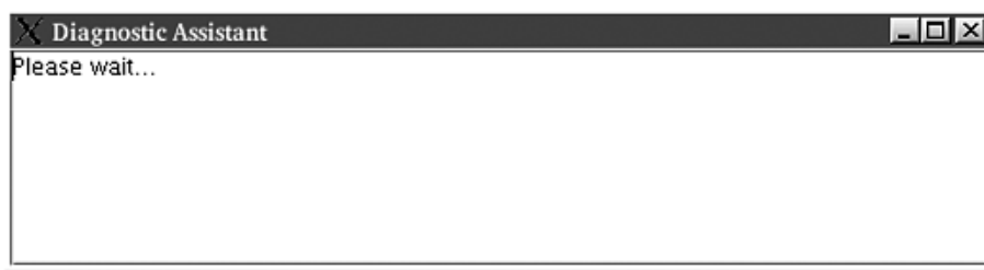
Figure 13.2 Application window with an added JTextArea for displaying questions
