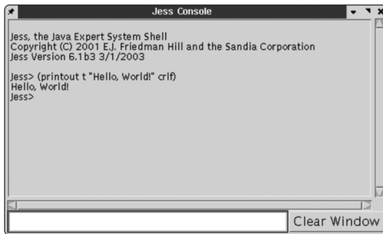
Figure 3.1 The Jess.Console interface for Jess. This as an alternative to the command-line Jess.Main interface. You can enter Jess code in the small text field at the bottom left, and Jess output appears in the scrolling text area at the top.
