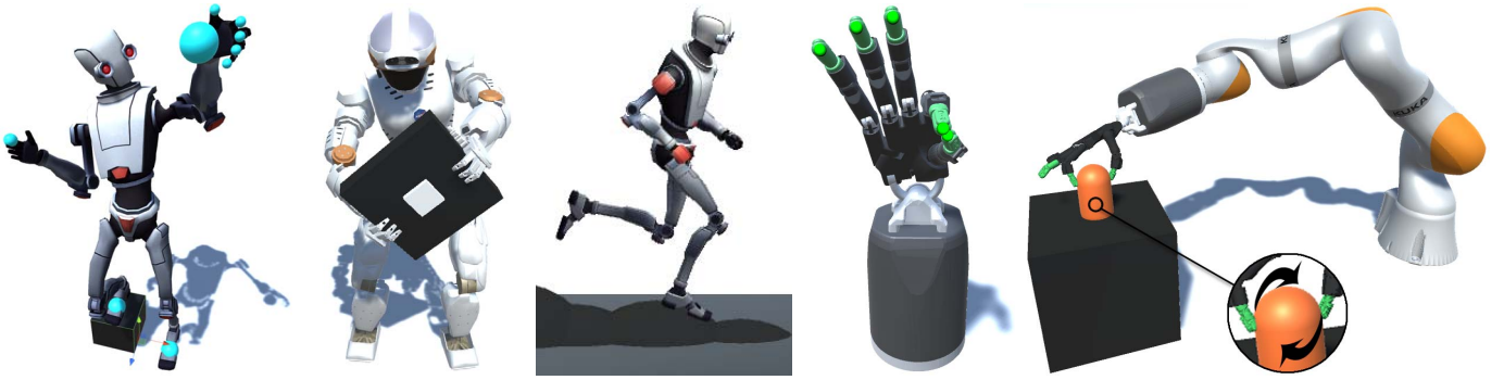
Fig. 2. Proposed algorithm solving generic full-body inverse kinematics for different geometries and application scenarios.
