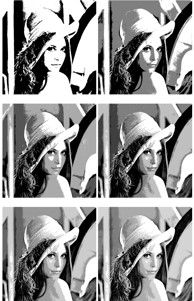
Fig. 5. Lena image thresholded by one to six thresholds from top left to bottom right, respectively using the proposed GbSA.
