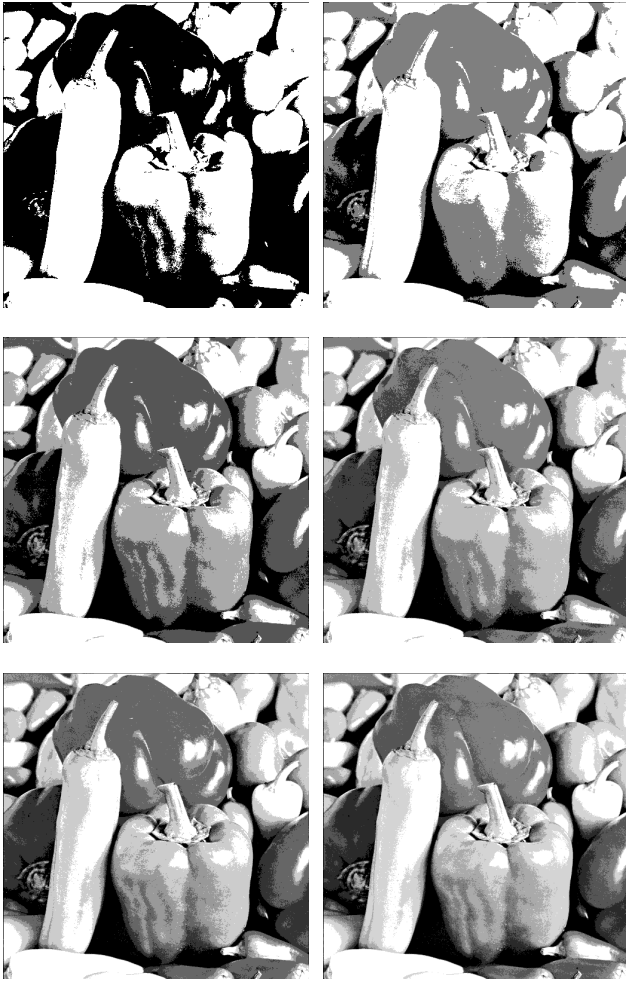
Fig. 6. Peppers image thresholded by one to six thresholds from top left to bottom right, respectively using the proposed GbSA.
