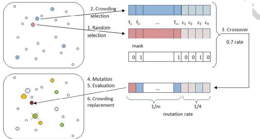
Figure 3: One iteration in MNC GA for unsupervised feature selection.
