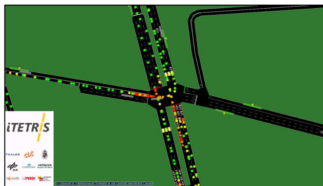
Figure 10. Speed information collection by RSUs. Each dot represents one data point, the color represents the speed (green means fast, red slow).
