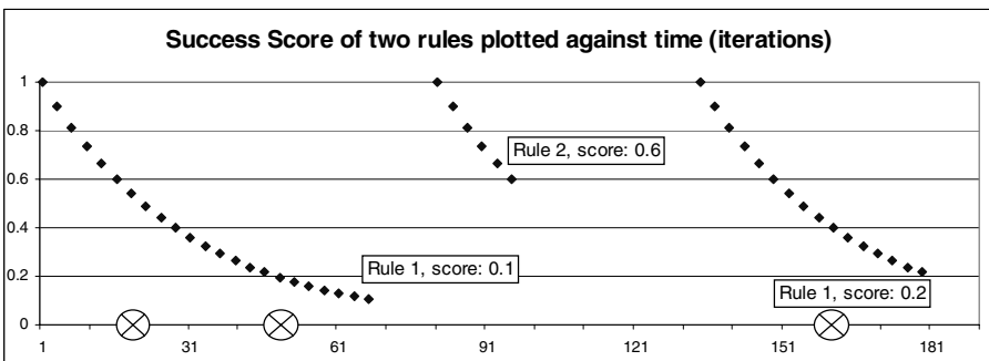
Figure 19-1. This is an example of the success scores of the execution of two rules. The ⊗ sign along the X-axis marks re-applications of the action of the rule before the search manages to arrive at the desired outcome. Here, Rule 1 is executed twice. The scores of 0.1 and 0.2, which is normalized over two executions to obtain NSS of 0.15, imply that either the strategy or the formulation of desired outcome adopted in Rule 1 has problem; whereas the high NSS of 0.6 of Rule 2 implies the potential effectiveness of the strategy used in Rule 2. These rules will then be applied to other training instances to obtain ANSS.
